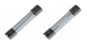
3AG type fuse used in control cabinets. Good (left), Blown (right). The wire in the 3AG fuses is visible through the glass casing and it is easy to tell if the fuse is blown.
