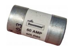
HRC fuse used in village distribution. HRC fuses are filled with sand to stop the current arcing when the fuse blows. It is not always visibly obvious that the fuse has blown.
